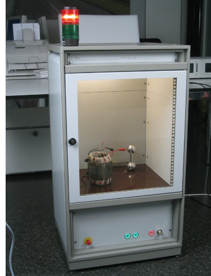
Partial discharge test cabinet for stator coils of small induction motors
