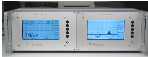
Partial discharge test cabinet for stator coils of small induction motors
