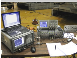
Advanced PD test system
